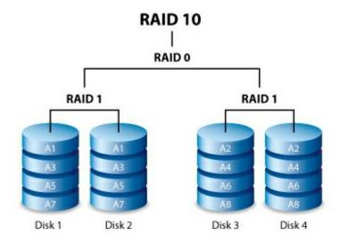
RAID 10 is a great choice for database managers that need to read and write a multitude of smaller files across the array's disks. The impressive IOPS and data protection offered by RAID 10 gives database managers impressive reliability both in keeping files safe and rapid access.
