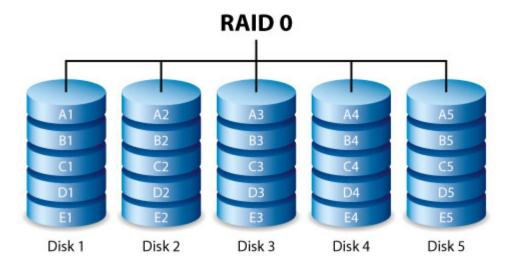
However, RAID 0 lacks a very important feature: data protection. If one hard drive fails, all data becomes inaccessible. A recommended option is RAID 5, which offers:
