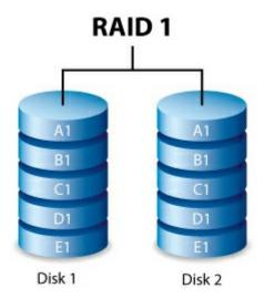
However, due to the time it takes to write data multiple times, performance is reduced. Additionally, RAID 1
