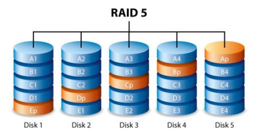
While the files stored on a RAID 5 array remain intact should one hard drive fail, data can be lost if a second hard drive fails before the RAID is rebuilt with the replacement hard drive.
