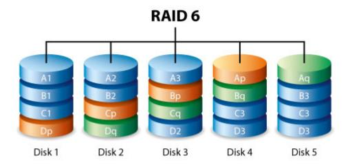
RAID 6 synchronizing from a failed disk is slower than RAID 5 due to the use of double parity. However, it is far less critical due to its double-disk security.
