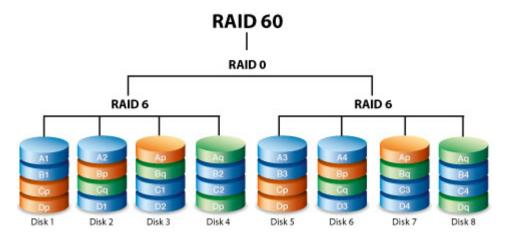
Since a RAID 60 array has a high number of hard drives, the time to initialize and rebuild data is longer than a single RAID level.
