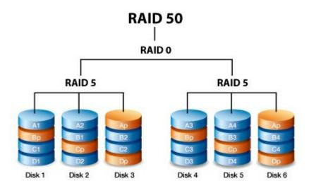
A RAID 50 array with a high number of hard drives increases the time to initialize and rebuild data due to the large storage capacity.
